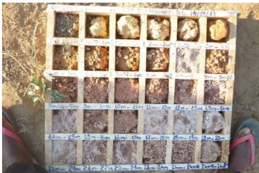
Soil samples taken during drilling
