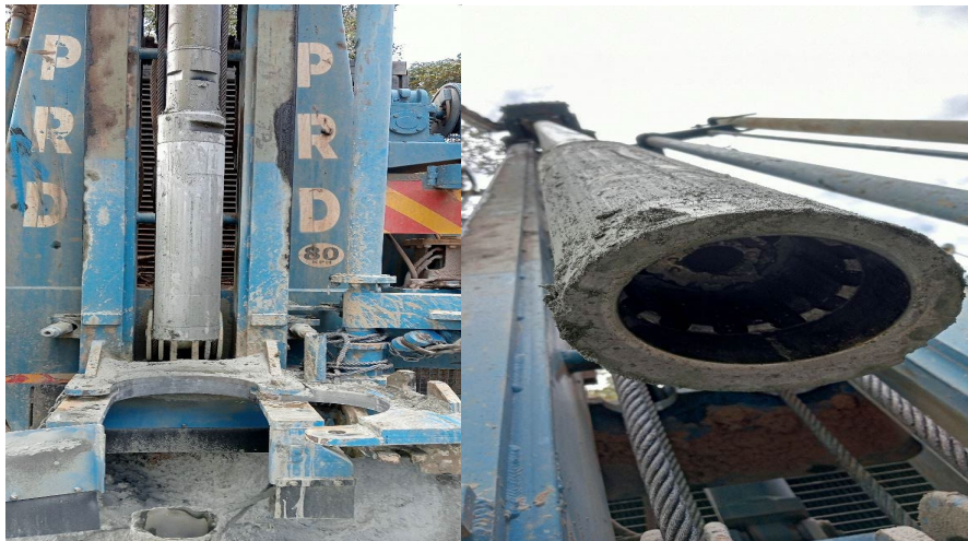
Hammer with a broken bit
