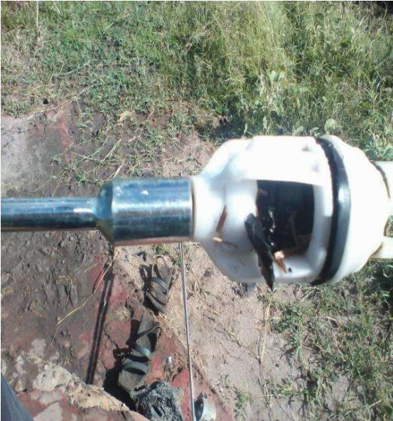
A faulty foot valve can render a pump useless.
